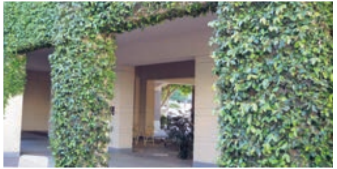
Vegetative screening can be used to reduce solar heat loading.
