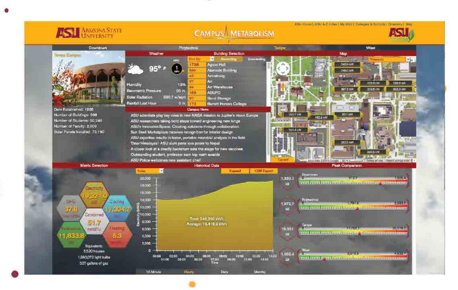
The initial overview allows an instant window into how a campus or building is performing. The data displayed shows metrics on electrical, cooling and heating usage as well as overall greenhouse gas emissions and renewable energy production.
