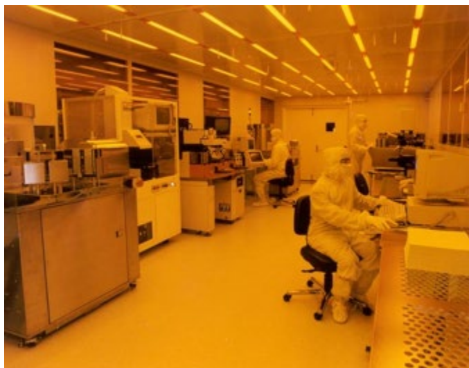
Figure 5- Typical photolithography bay with yellow/amber lighting
