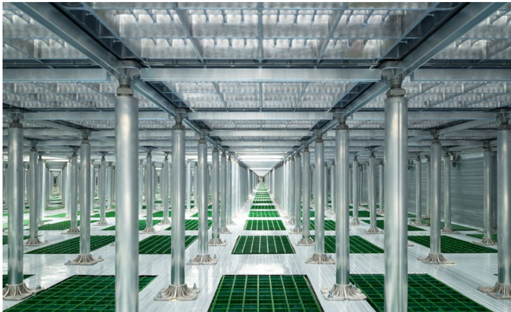
Figure 19- Raised Access Flooring System with 24 x 24 in Panels and Grates with Corner Locks and Continuous Stringers
