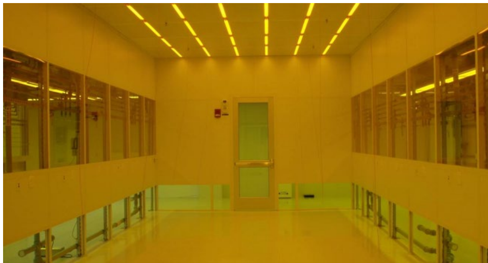
Figure 24- Typical Photolithography Bay with Yellow/Amber Lighting and Window Tinting
