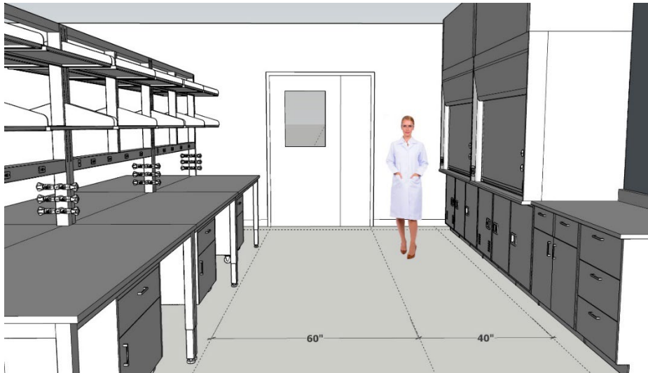
Diagram 4: Fume Hood Distance to Lab Casework when Located in an Exit Access
