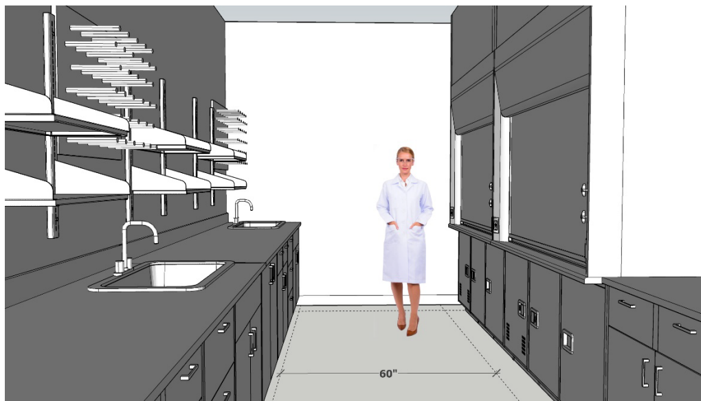
Diagram 8: Fume Hood Distance to Lab Casework when Located in a Lab or Lab Support Room
