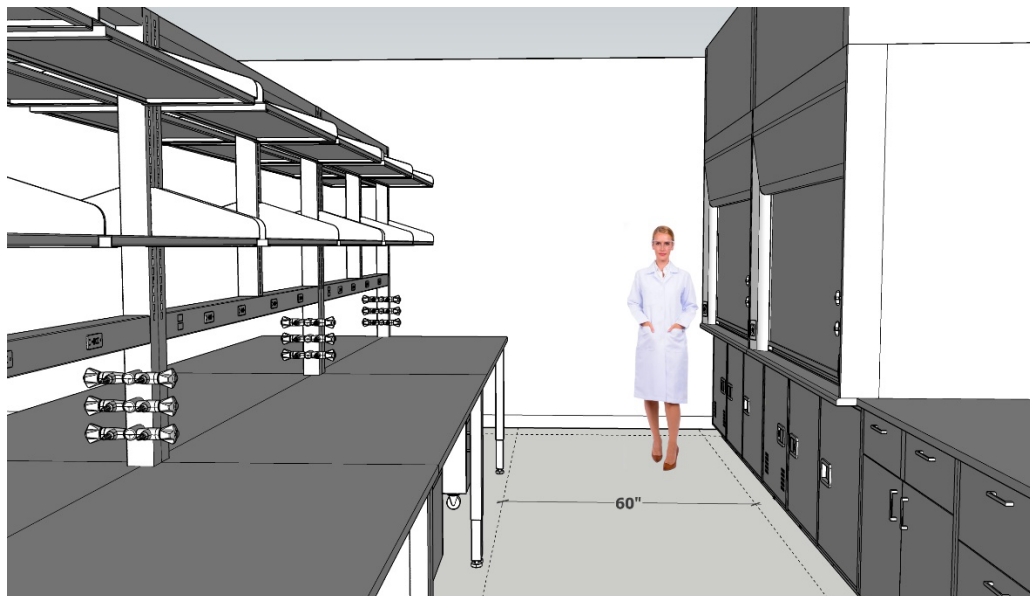
Diagram 7: Fume Hood Distance to Open Lab Benches when Located in the Back of a Lab
