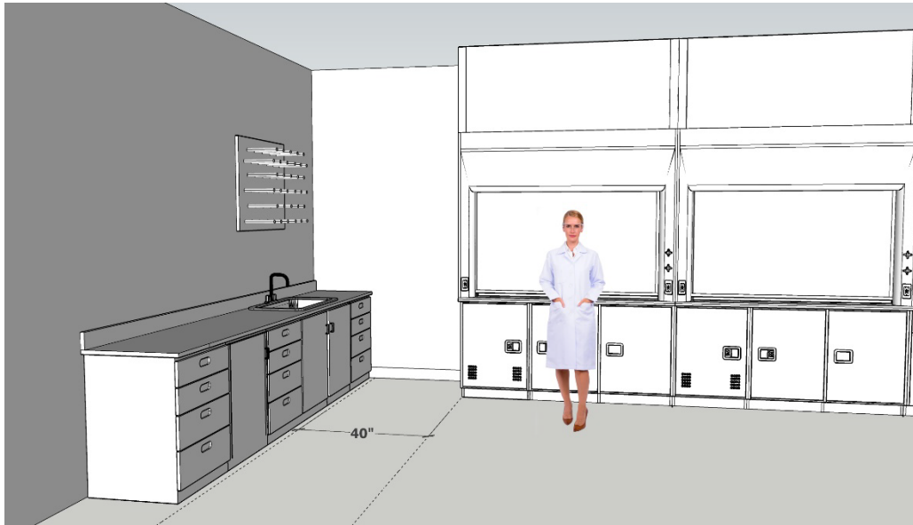
Diagram 2: Fume Hood Side Distance to Face of Side Lab Casework
