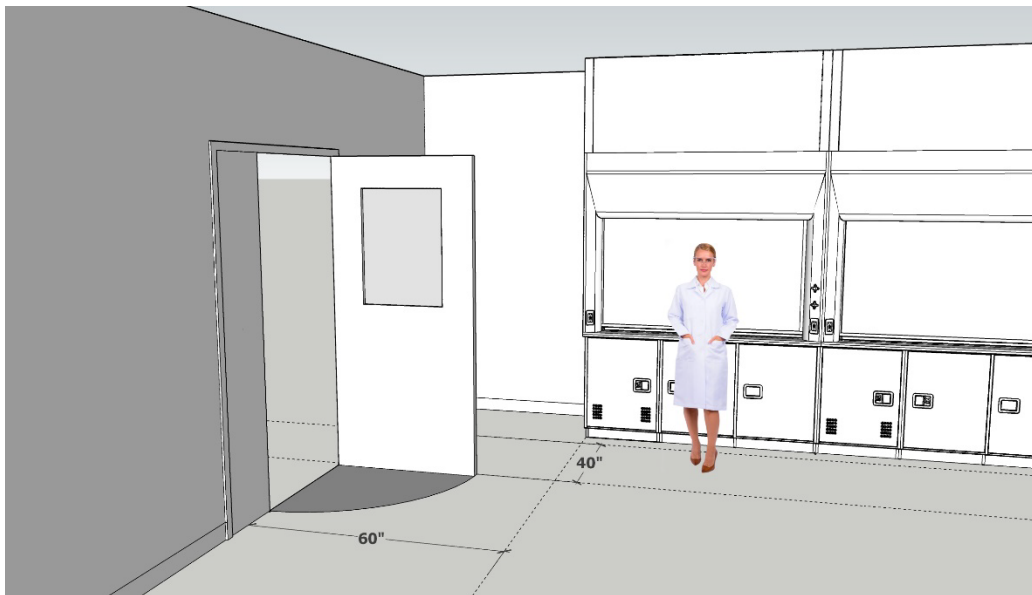
Diagram 5: Fume Hood Distance to Door Opening or Framed Opening Toward the Side of a Fume Hood
