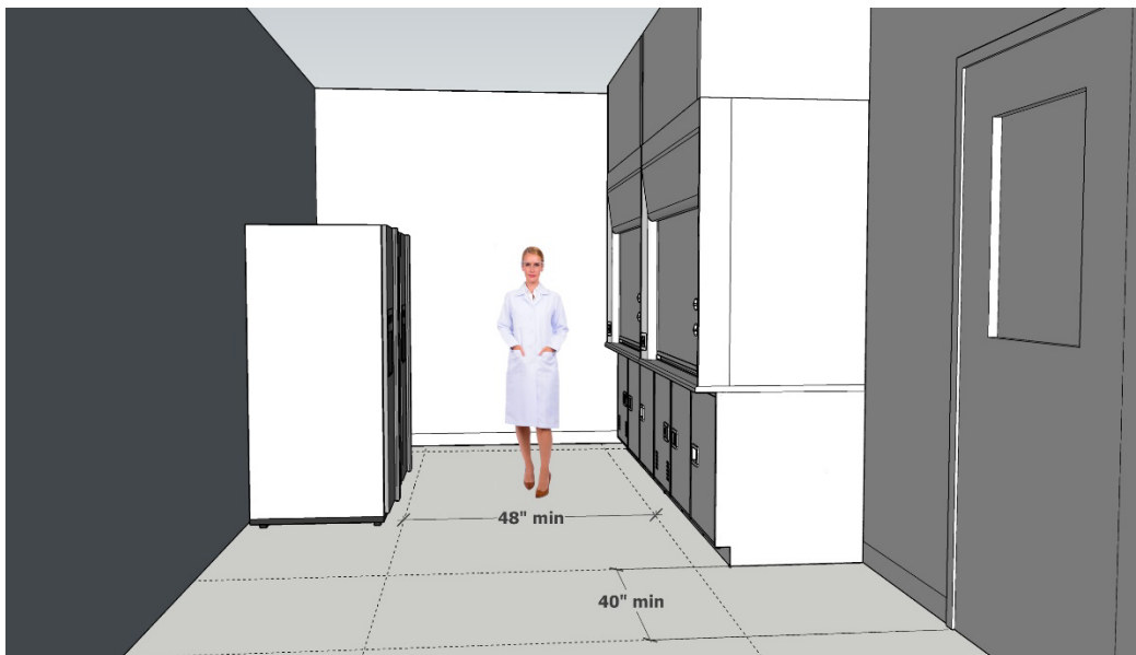
Diagram 3: Fume Hood Distance to Lab Equipment
