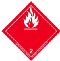
Department of Transportation warning placard: Category 2, flammable gas.
