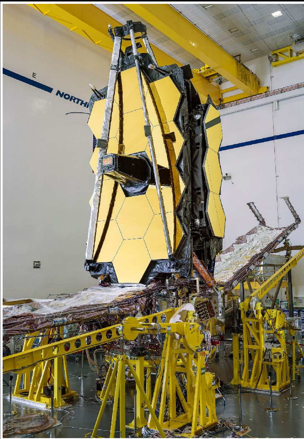
August 2019: JWST OTE+ISIM integrated with Sunshield+Spacecraft!
