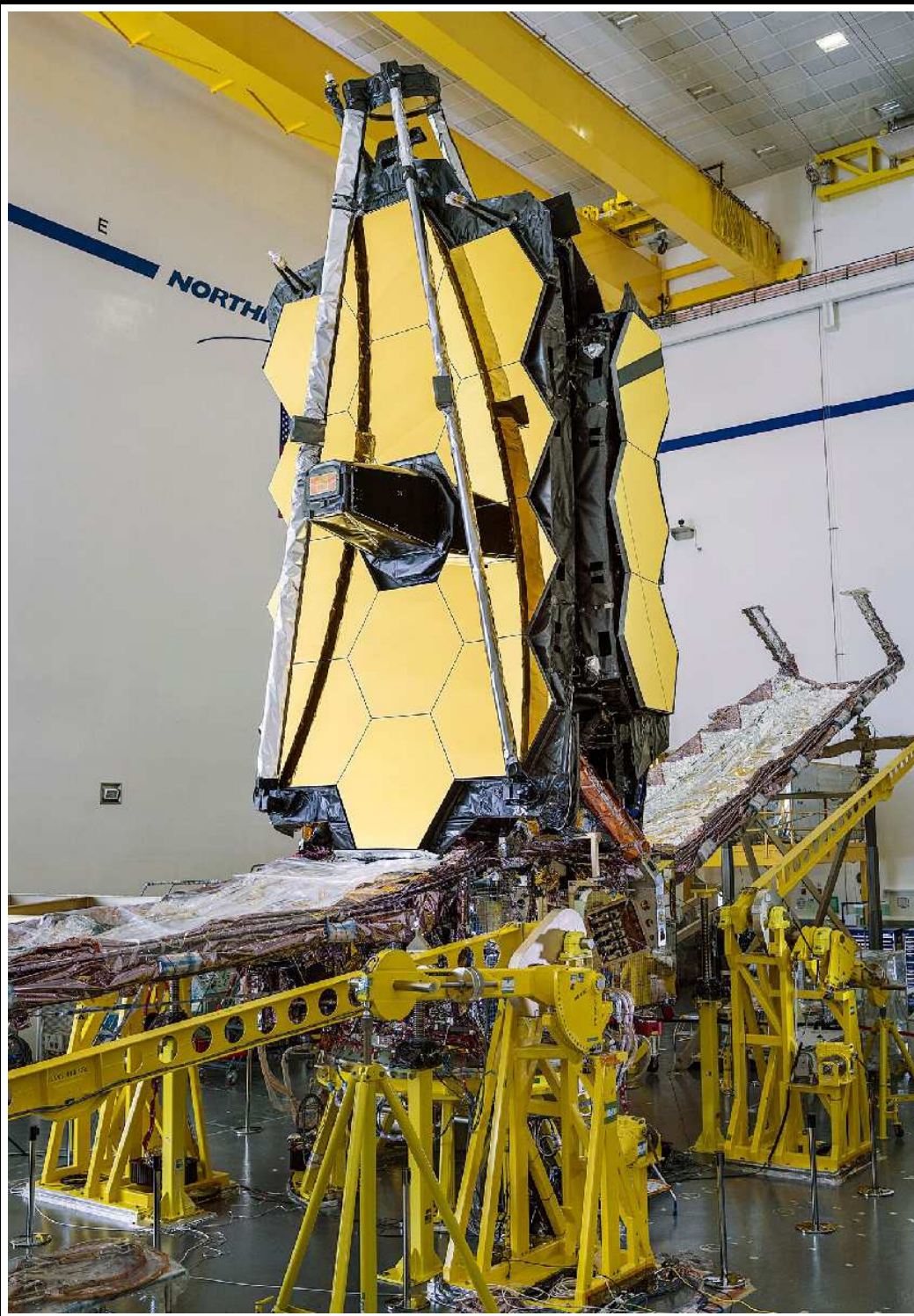
August 2019: JWST OTE+ISIM integrated with Sunshield+Spacecraft!
