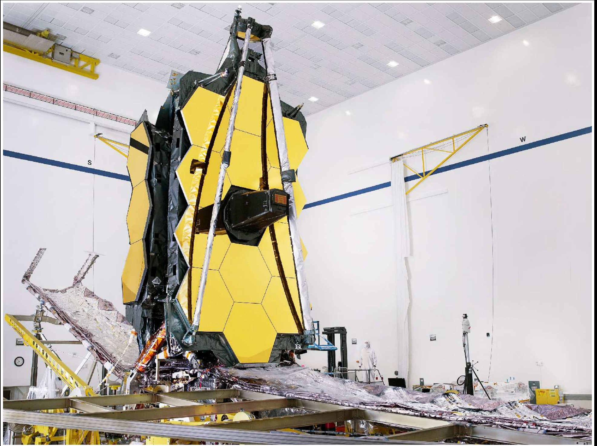
August 2019: JWST OTE+ISIM integrated with Sunshield and Spacecraft!
