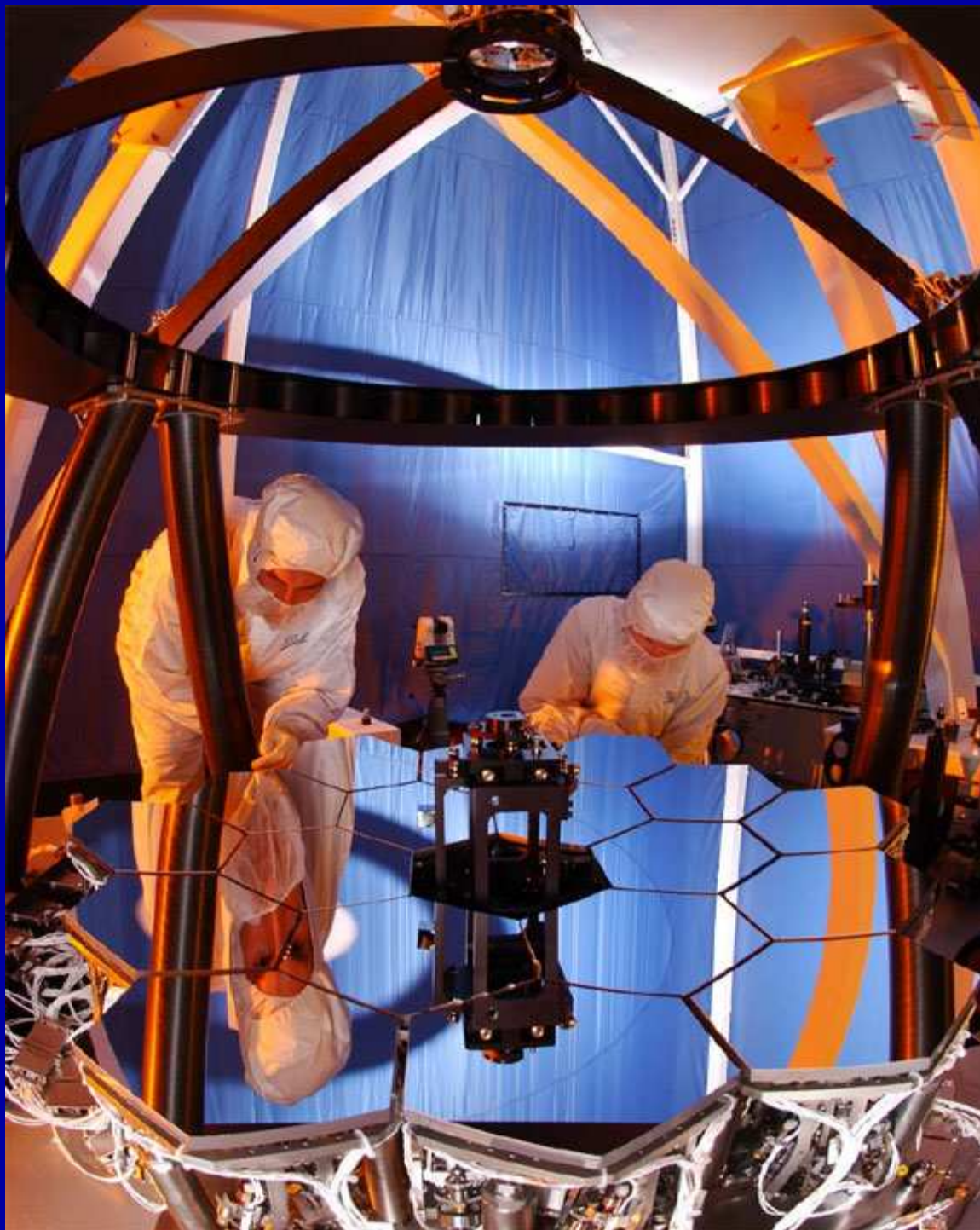
Ball 1/6-scale model: WFS produces diffraction-limited images at 2.0\ \mu\text{m} .
