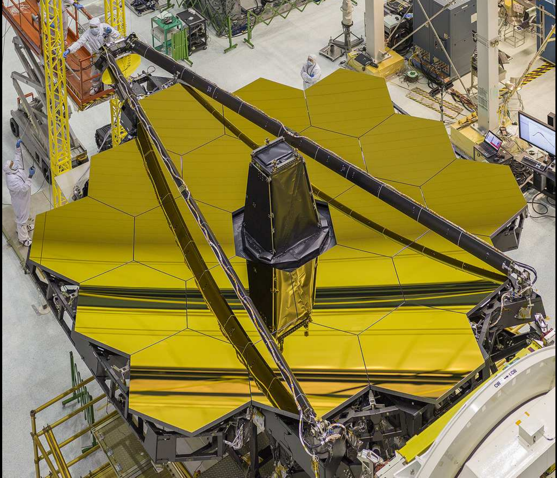
JWST stowed for further instrument mounting
