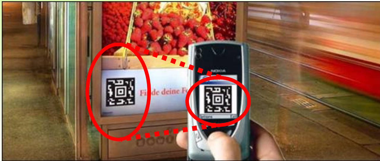
Camera Phone Acquiring Image of 2 Dimensional Bar Code and Linking Mobile Handset to Advertiser's Web Site Source: Neomedia Technologies
