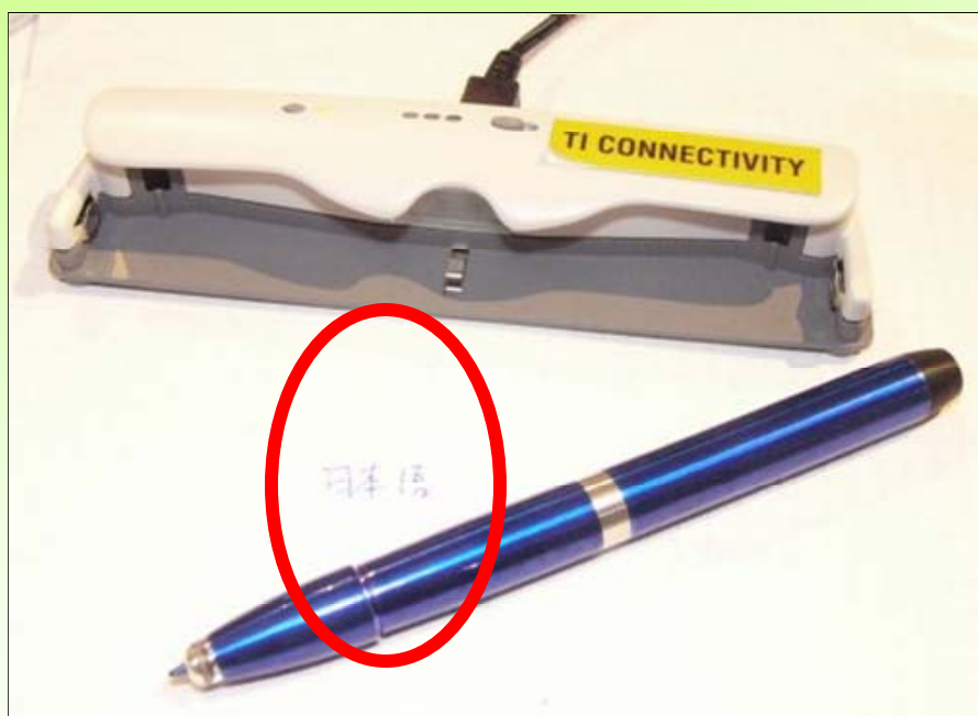
Optoelectronically-Enabled Handwriting Input Device for Delivering Text and Drawings to Wireless Handset Source: CandleDragon, Inc.
