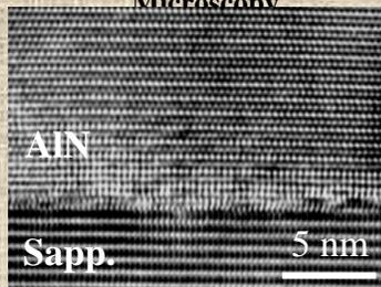
Cross-sectional electron micrograph showing misfit dislocations at sapphire/AlN interface.
