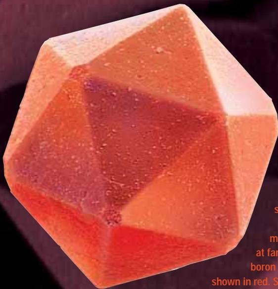
Lawrence Garvie used a scanning electron microscope to obtain images of  $B_2O_3$ . The molecular structure is modeled at far right. Small knobs represent boron with the larger oxygen atoms shown in red. SEM pseudocolor image at left shows a single 20-sided symmetrical icosahedron.
