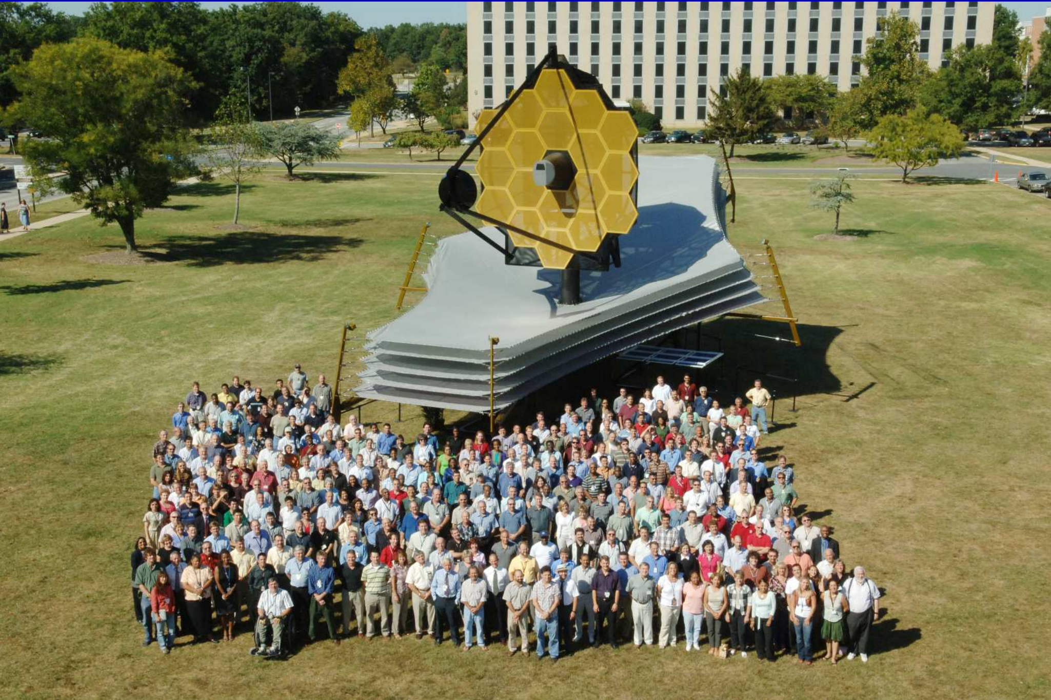
Life-sized model of JWST, used to test the deployment of its sun-shield.
