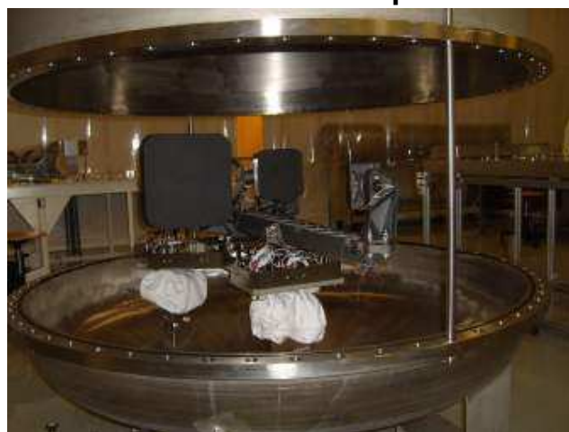
NIRSpec Fore Optics Mirror Assembly
