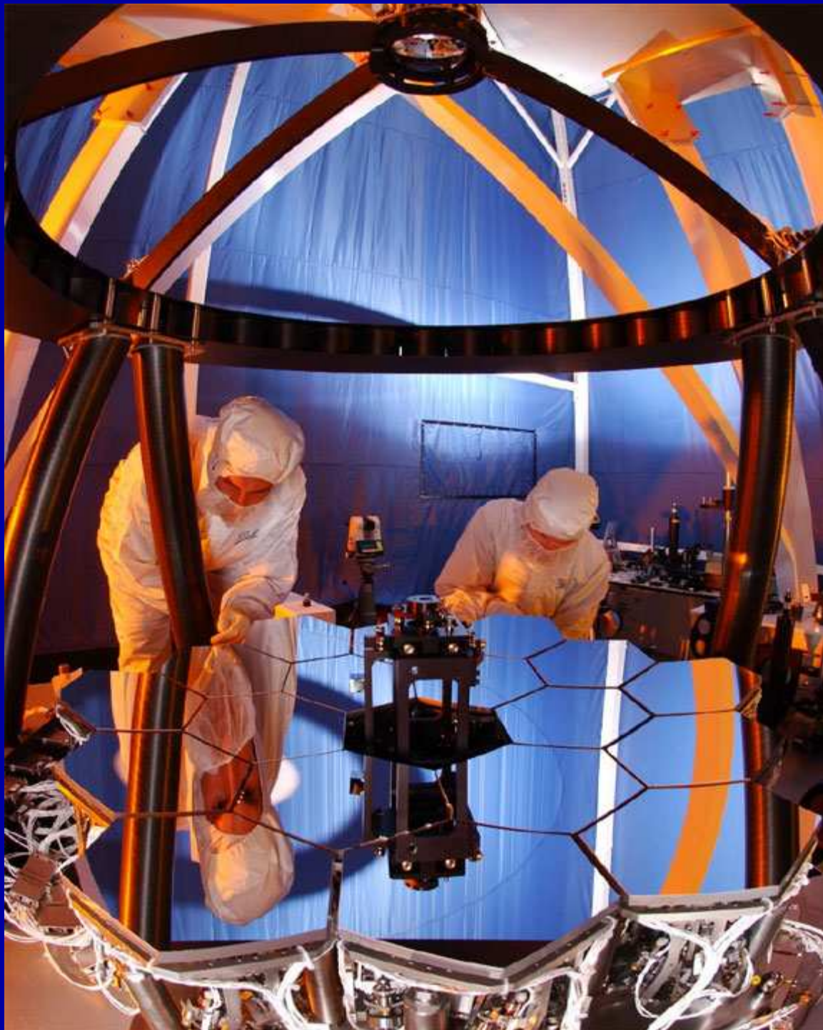
Ball 1/6-scale model: WFS produces diffraction-limited images at 2.0 \mu\text{m} .
