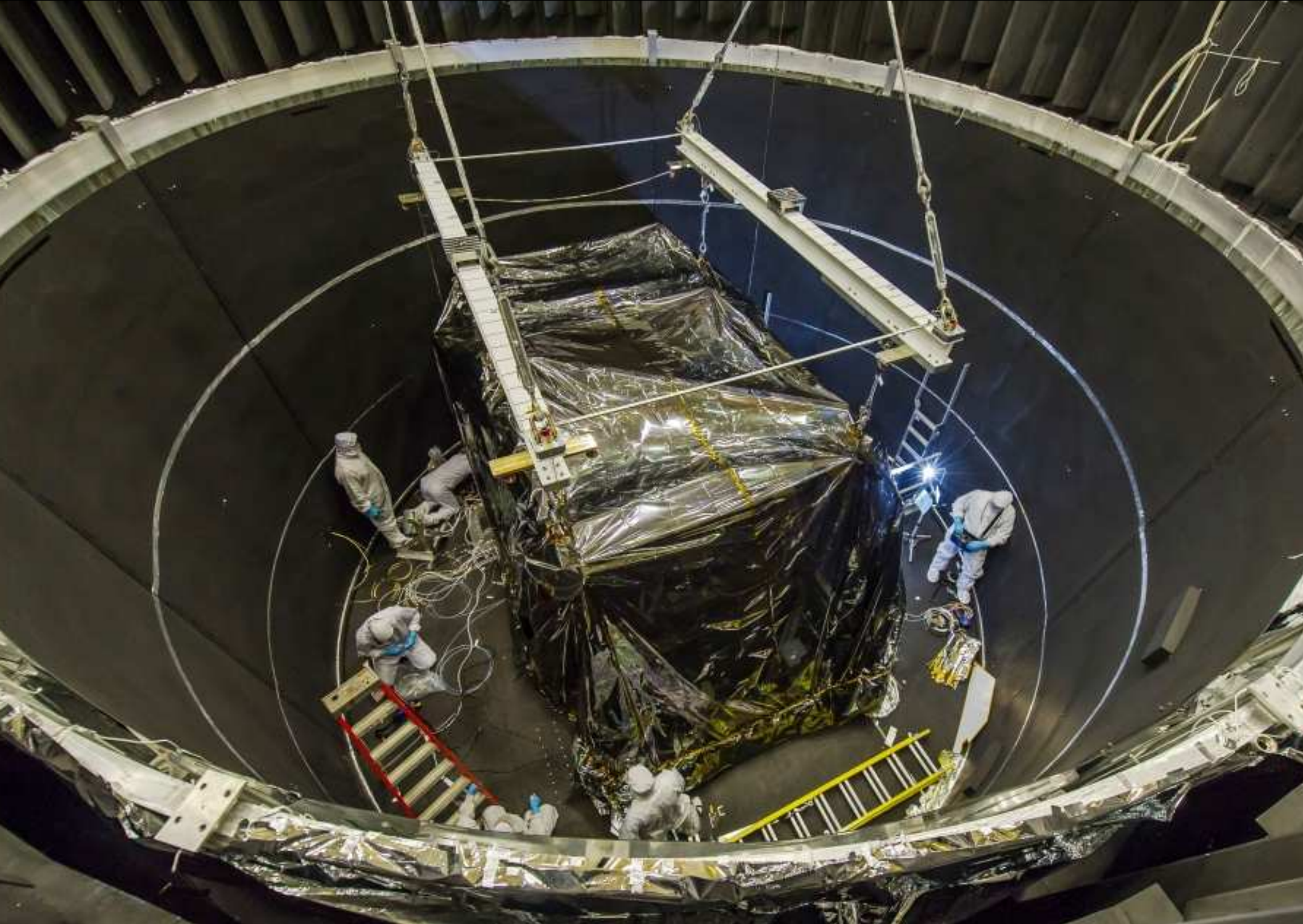
Aug. 2013: Actual Flight ISIM (with MIRI and FGS) lowered into OSIM.
