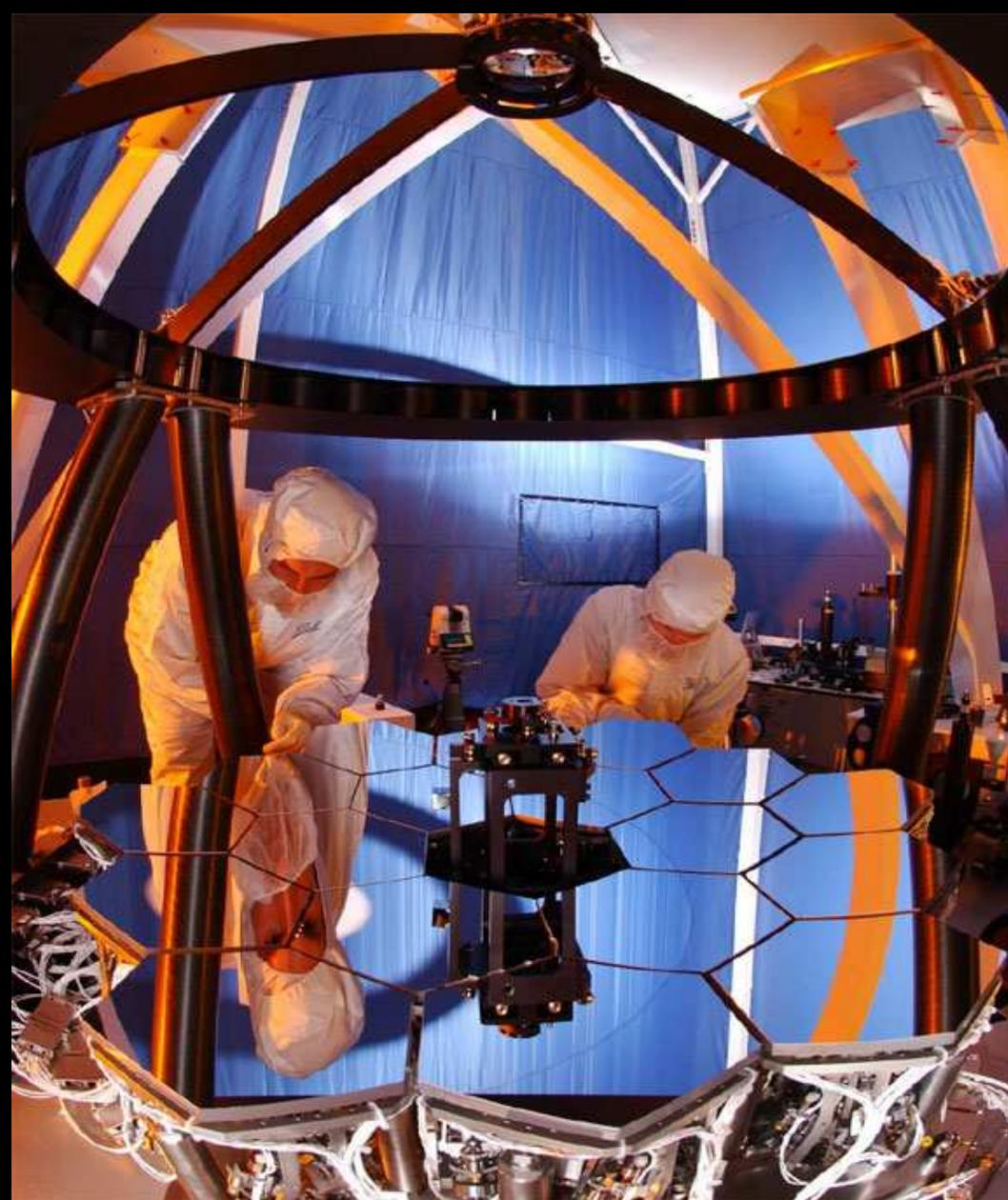
Ball 1/6-model for WFS: diffraction-limited  $2.0 \mu\text{m}$  images ( $\text{Strehl} \gtrsim 0.85$ ).
