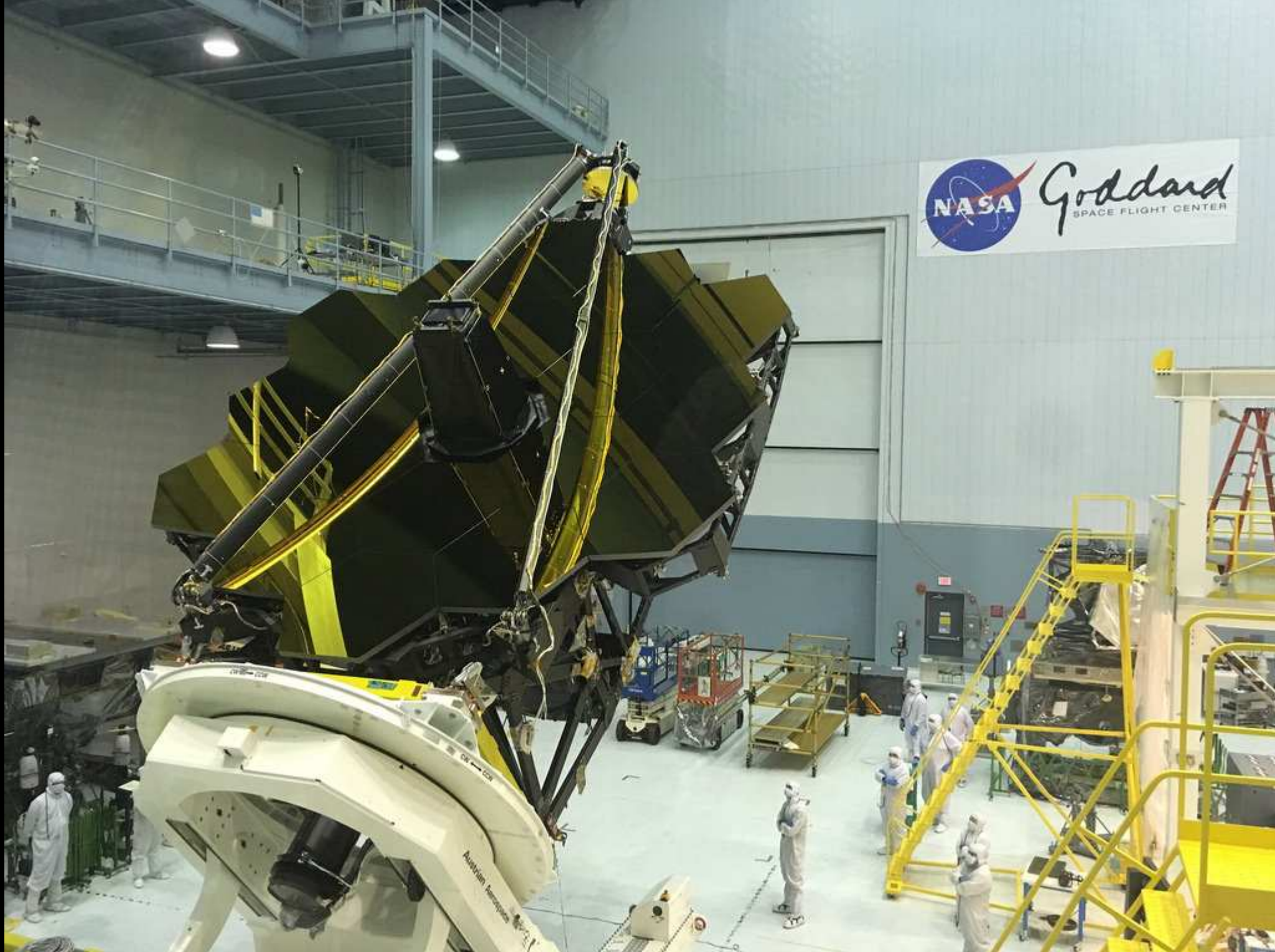
JWST being tilted into the right position
