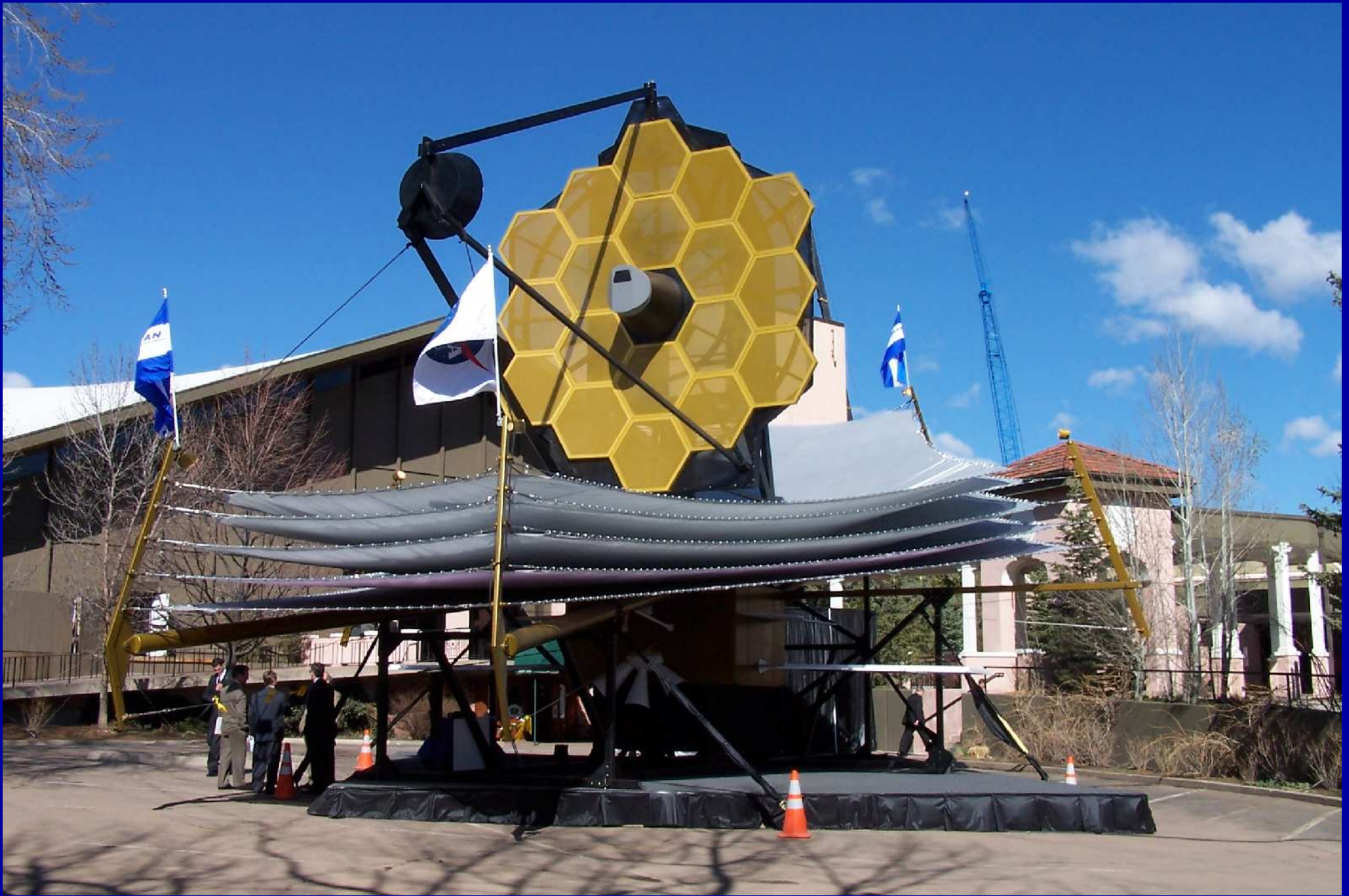
A life-sized model of JWST, used to test the deployment of its sun-shield.
