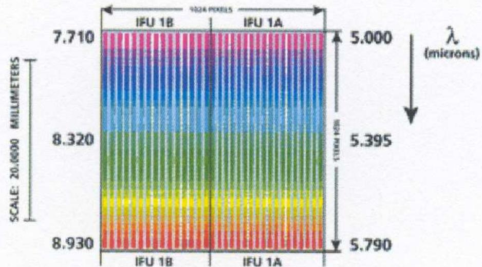
Figure 50. Schematic illustration of the MIRI IFU image slicer format (left) and dispersed spectra on detector (right)
