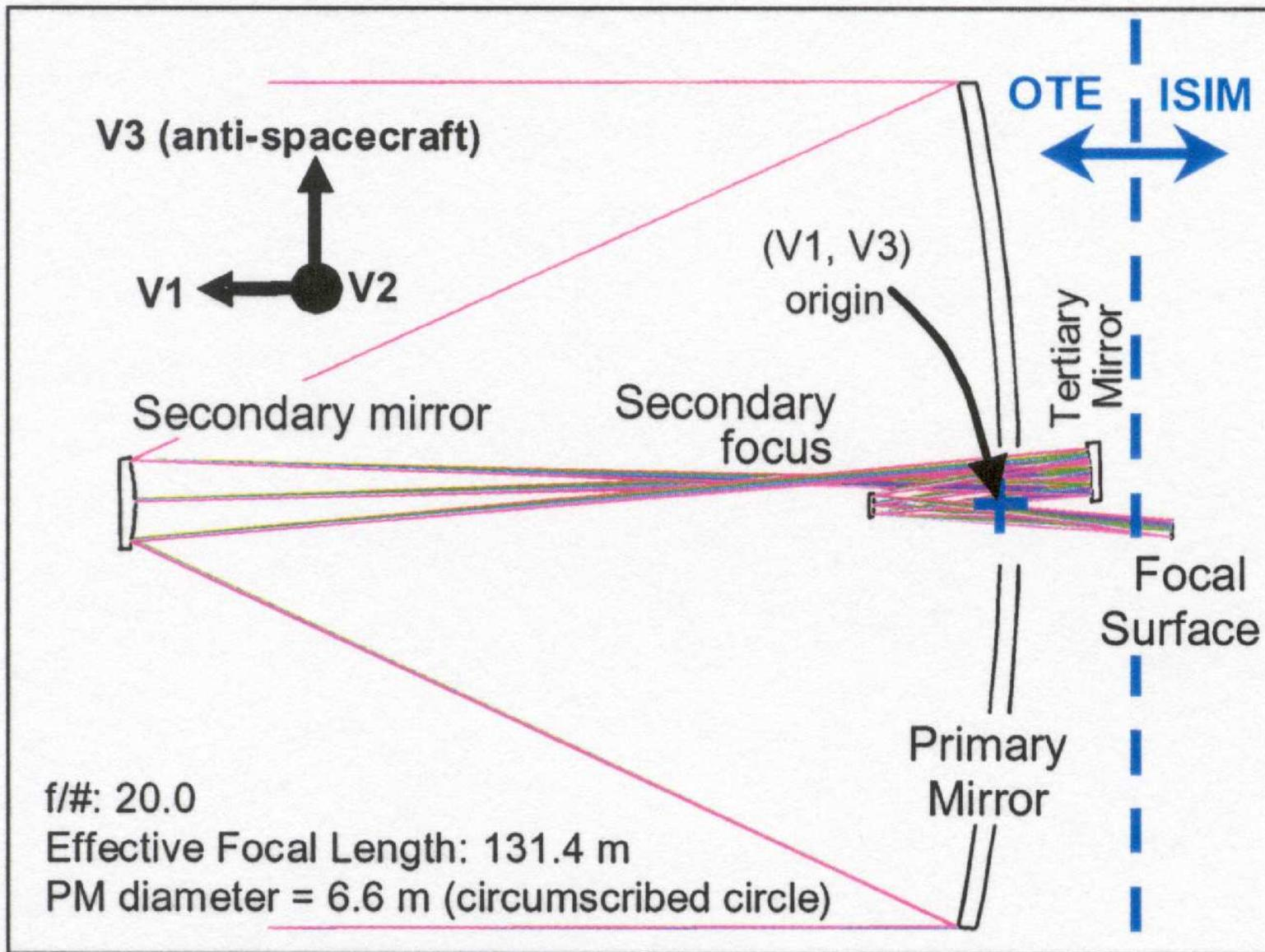
Figure 33. OTE optical layout
