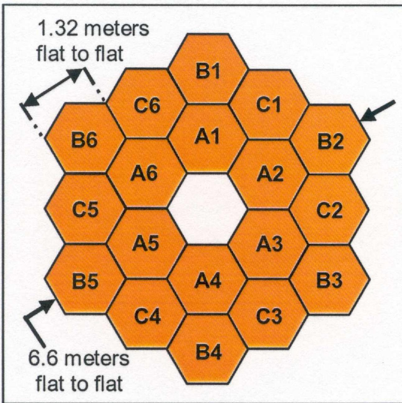
Edge-to-edge diameter is 6.60 m, but effective circular diameter is 5.85 m.
