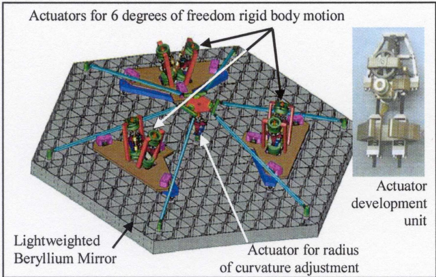
Figure 36. Rear view of a primary mirror segment.
