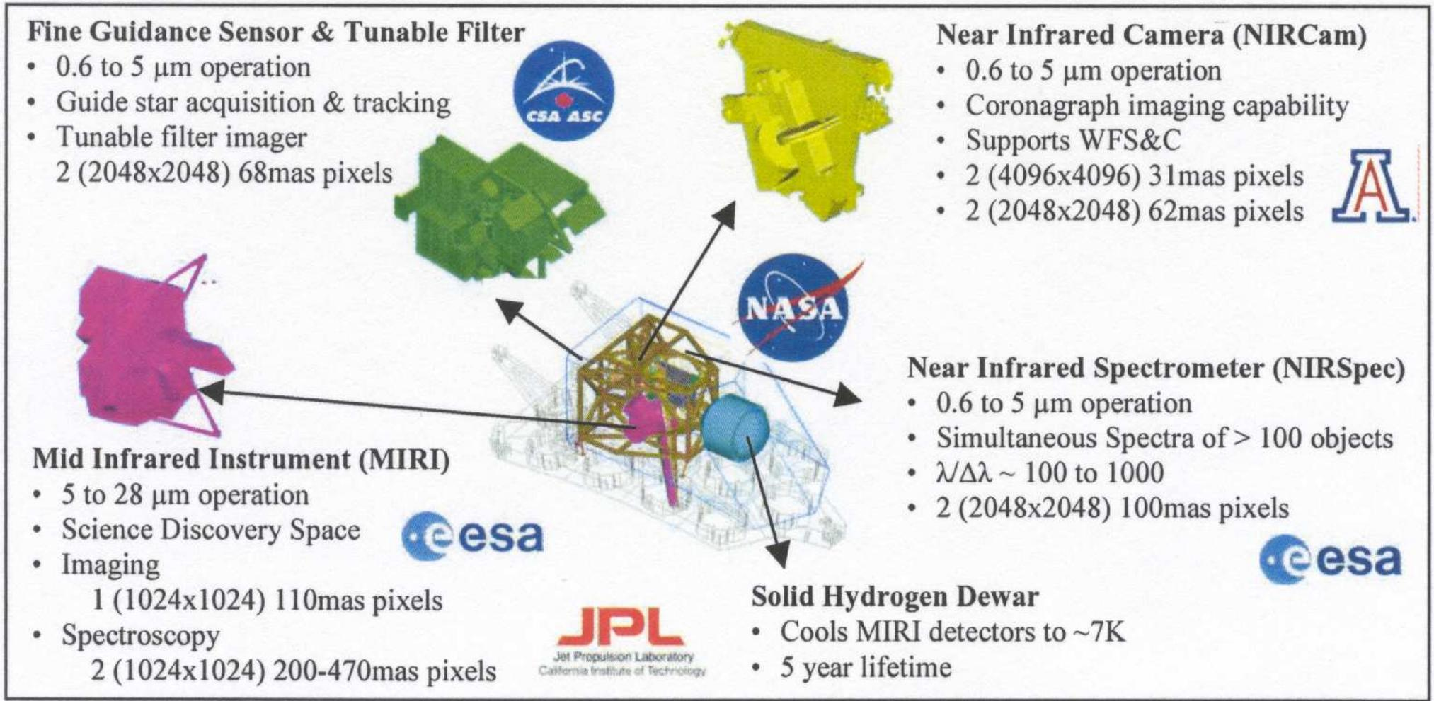
Figure 37. ISIM element and its science instrumentation.
