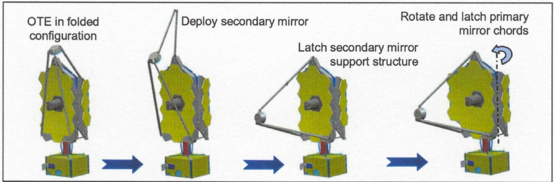
Figure 53. Telescope Deployment Sequence (Deployment steps 4 and 5)
