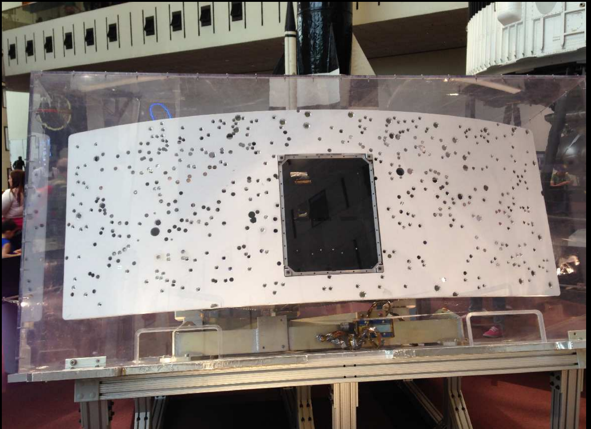
Hubble's WFPC2 returned to Smithsonian in 2009: Results from 16 years of micro-meteorite hits ... (holes drilled in shield for sample analysis).
