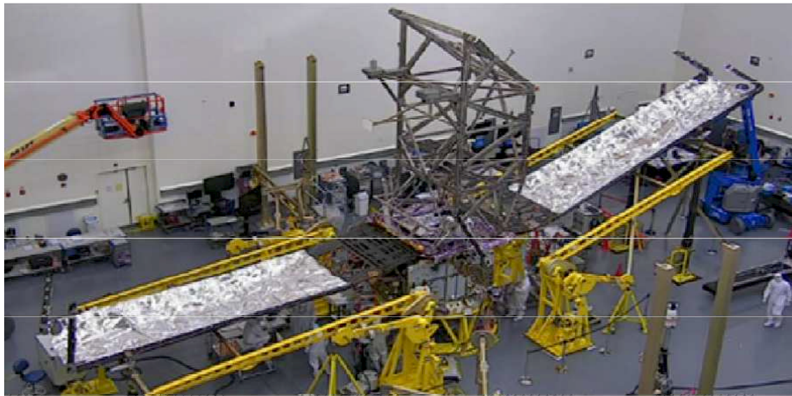
FWD/AFT UPSs Installed
