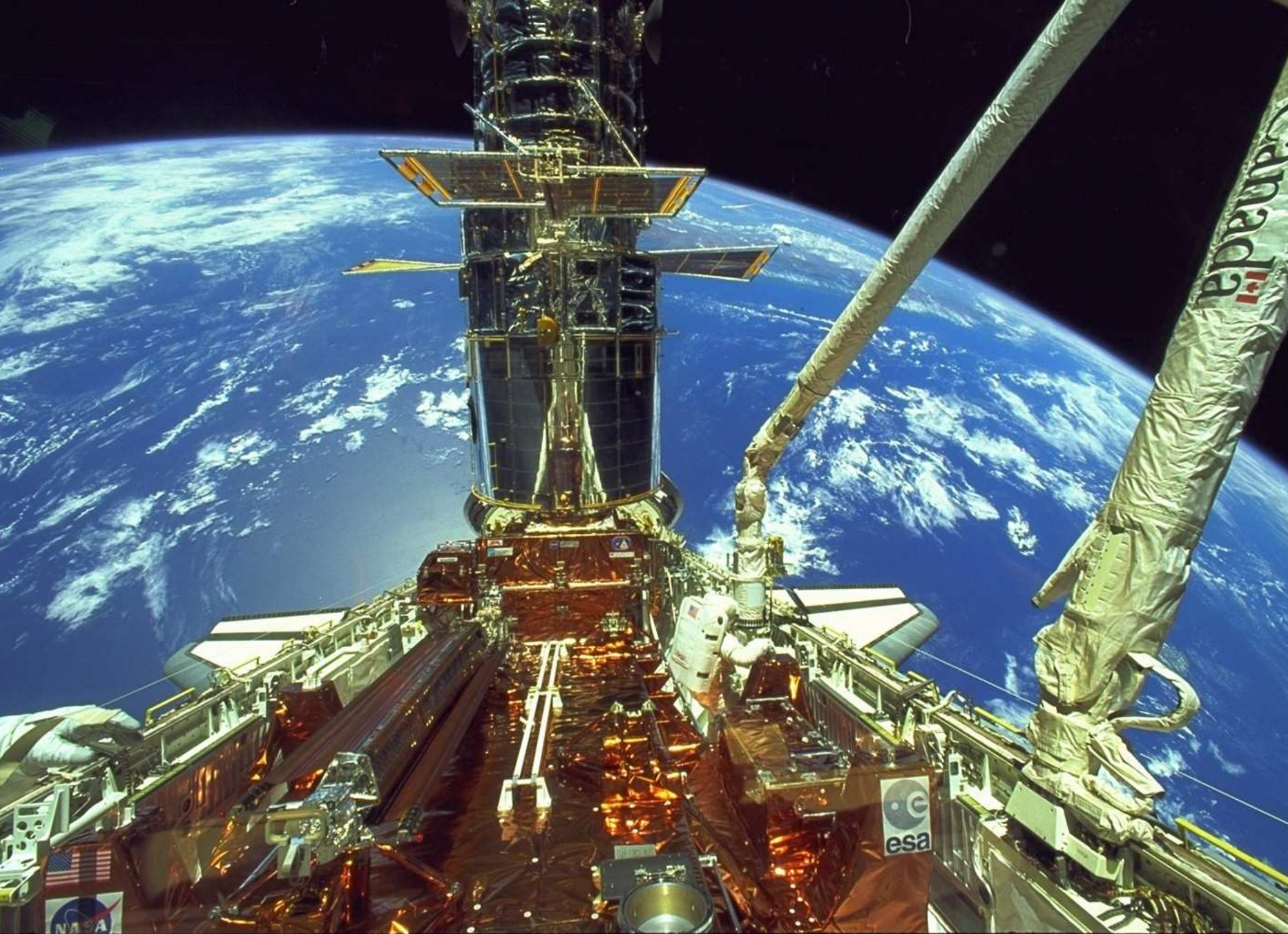
New ESA solar panels rolling out during SM1 in December 1993
