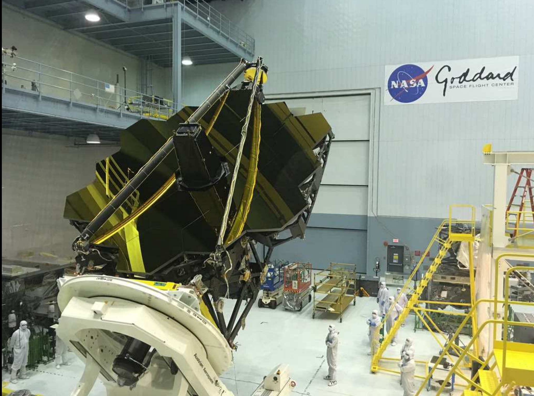
James Webb Space Telescope (JWST) tilted into the required position
