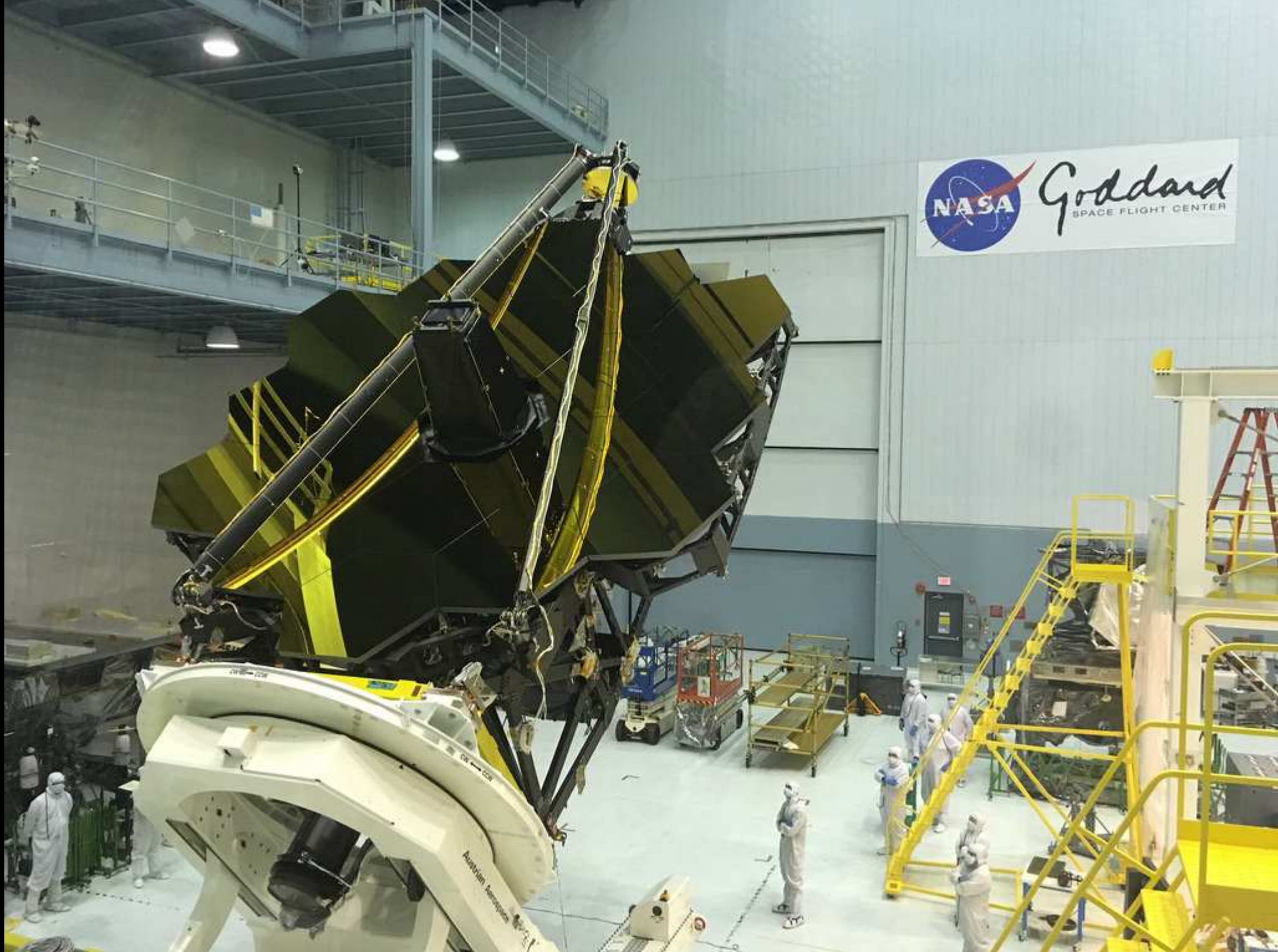
JWST being tilted into the right position
