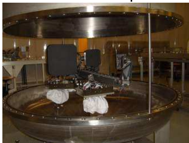
NIRSpec Fore Optics Mirror Assembly
