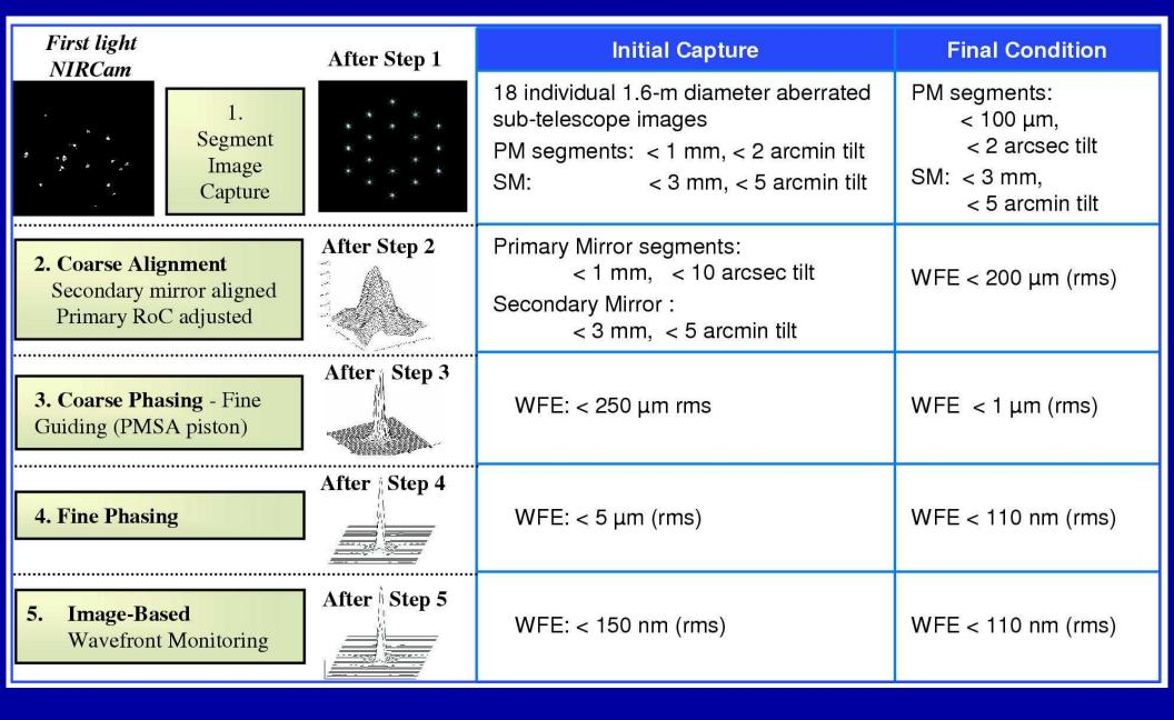
JWST's Wave Front Sensing and Control is similar to that at Keck and HET. Successful WFS demo of H/W, S/W on 1/6 scale model (2  $\mu$ m-Strehl $\gtrsim$ 0.85). Need WFS-updates every  $\sim$ 10 days, depending on scheduling/SC-illumination.
