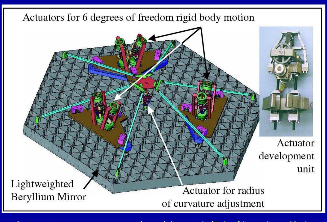
Active mirror segment support through hexapods (7 d.o.f.), similar to Keck. Redundant & doubly-redundant mechanisms, quite forgiving against failures
