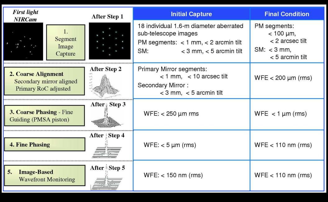
JWST's Wave Front Sensing and Control is similar to the Keck telescope. In L2, need WFS updates every 10 days depending on scheduling/illumination.
