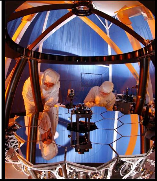
Wave-Front Sensing tested hands-off at 40 K in 1-G at JSC in 2013-2015.
