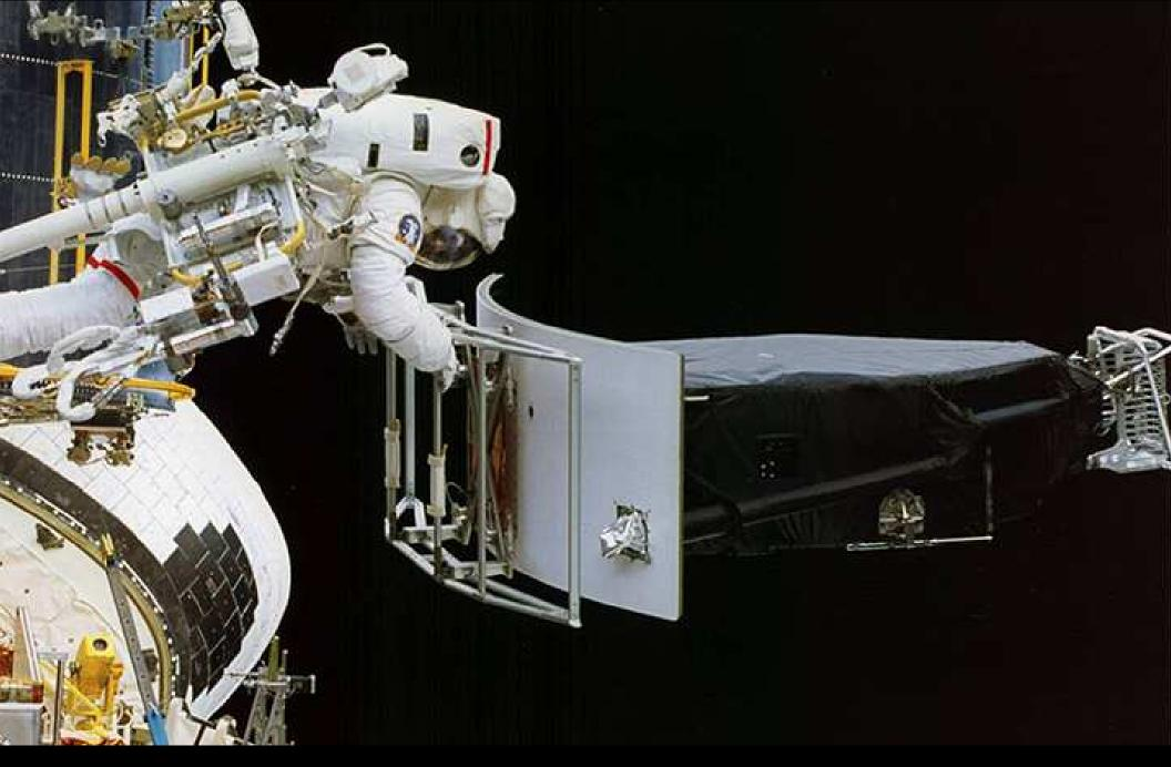
Installing Wide Field Camera 2 (WFPC2) during SM1 in December 1993. Similar to what astronauts did with WFC3 during SM4 in May 2009.
