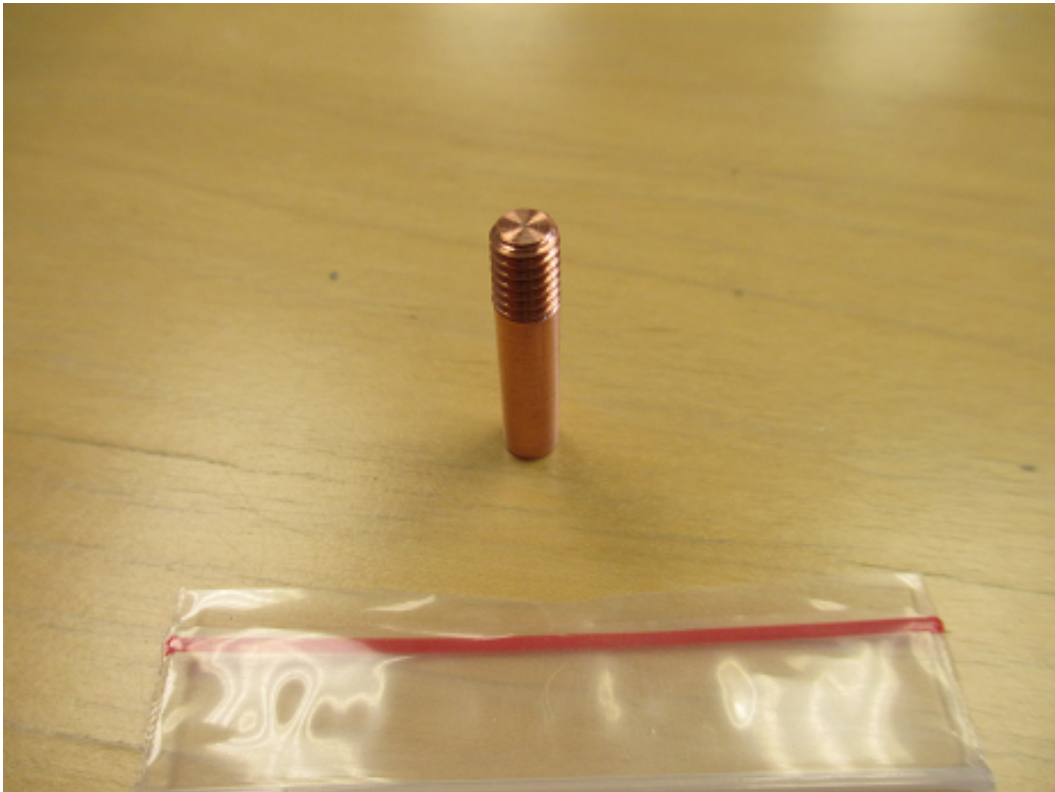
Figure 4.14: Copper support rod to serve as a guide pin and to maintain contact of the cold-head to the CCD during flight.
