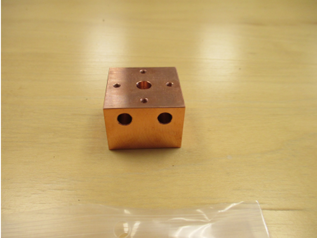
Figure 4.13: Copper cold-head interface to the CCD. The quarter-inch holes on the sides are for the heaters. The quarter-inch hole in the base is for the copper rod guide pin. The small 4-40 holes are for mating the cold strap.
