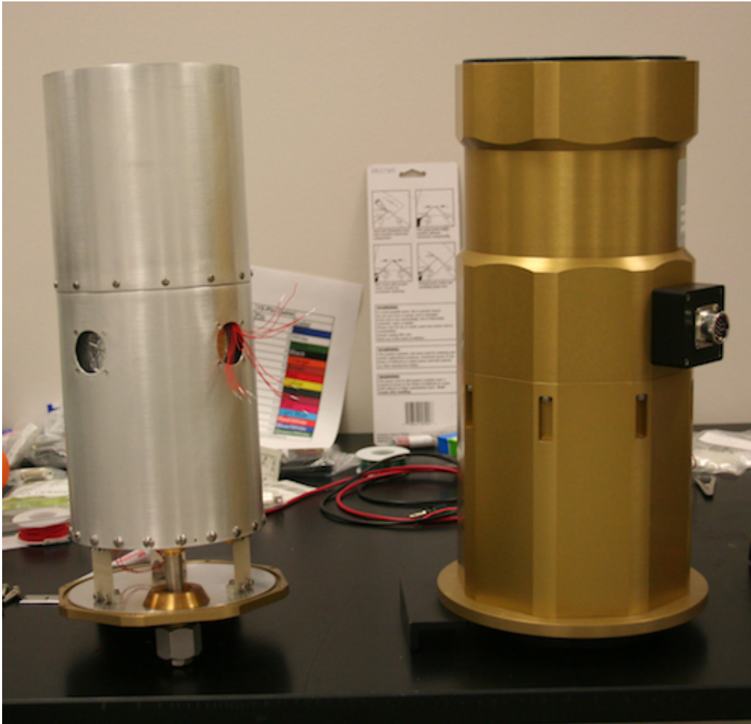
Figure 2.5: LASI facility CCD calibration dewar body shown disassembled.
