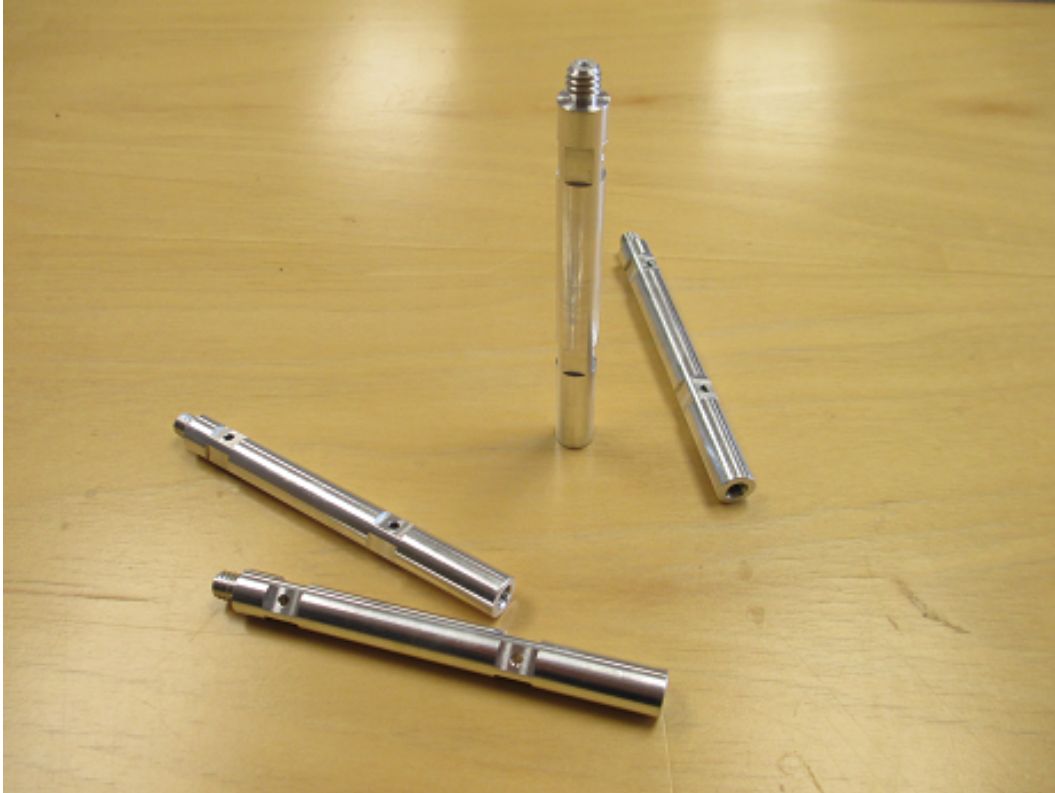
Figure 4.11: The Al7075-T6 aluminum support rods for maintaining rigidity throughout the rocket flight. The threaded end mates with the conflat mounting stage and the tapped end mates with the aluminum mounting stage.
