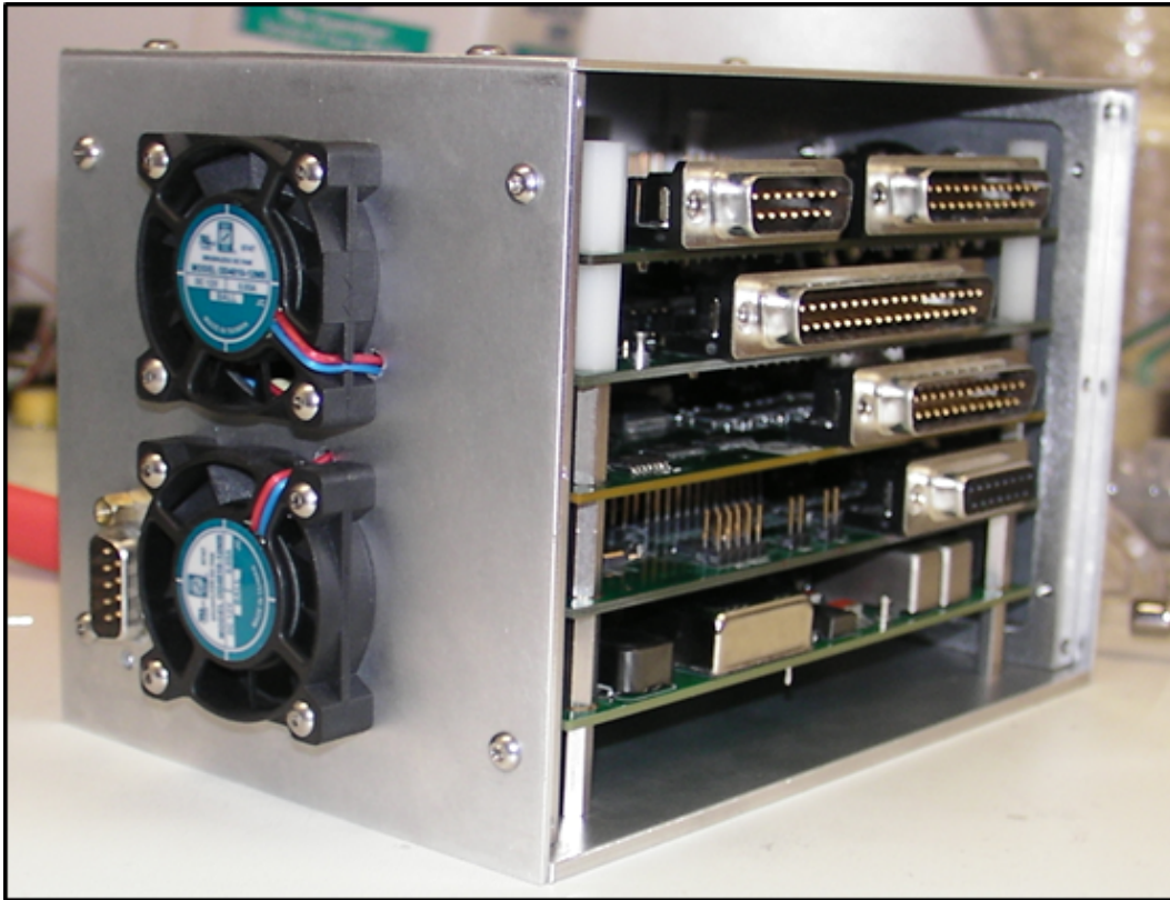
Figure 4.24: PCIe/104 Small-Cam imager controller from Astronomical Research Cameras, Inc. The fans on the side of the camera will not provide cooling during flight because forced air cooling is ineffective when there is a lack of air. A conductive cooling system will need to be developed in order to ensure the function of the Small-Cam in vacuo.
