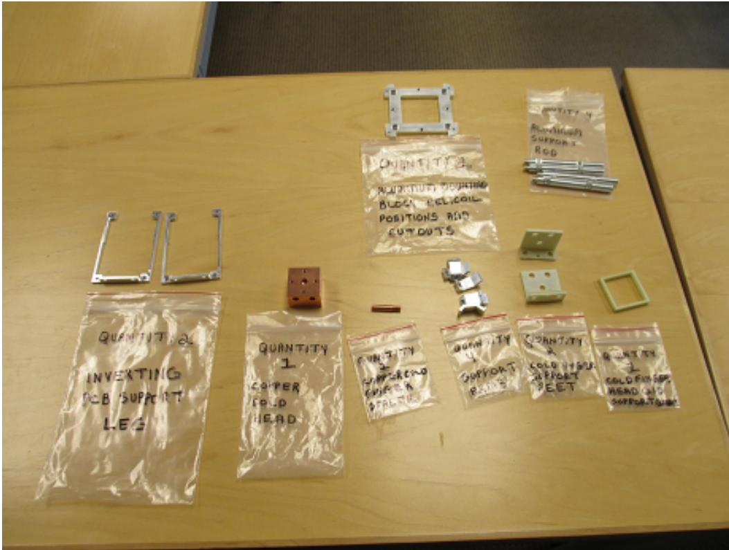
Figure 4.15: The machined parts for the rocket camera. On the left are the inverting board supports. The far right are the G10 materials that are provide thermal isolation of the cold surfaces from the neighboring components.
