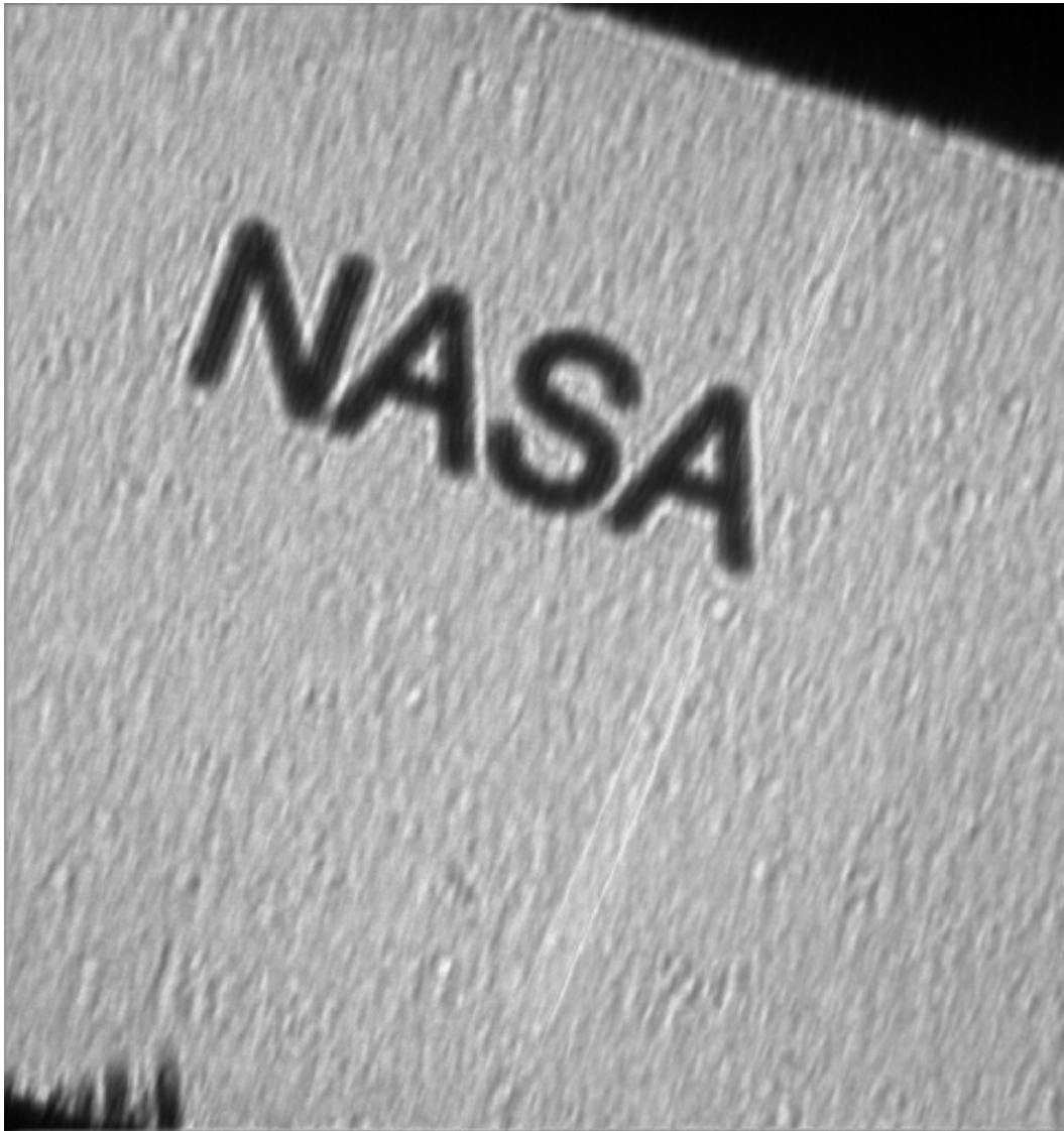
Figure 2.15: Sample reduced object frame that has been corrected for flat field variations and read noise for the small LBNL CCD. The mean signal level is \sim 32400 DN.
