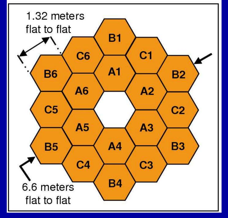
Edge-to-edge diameter is 6.60 m, but effective circular diameter is 5.85 m. Primary mirror segments are made (AxSys). Now being polished (Tinsley).
