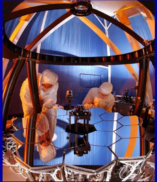
Ball 1/6-model for WFS: diffraction-limited 2.0  $\mu$ m images (Strehl $\gtrsim$ 0.85). Wave-Front Sensing tested hands-off at 45 K in 1-G at JSC in 2011-2013. In L2, WFS updates every 10 days depending on scheduling/SC-illumination.
