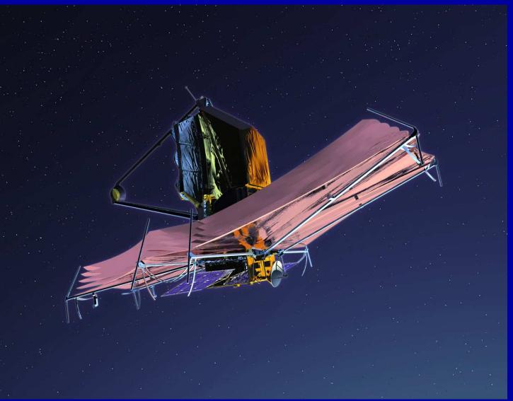
• A fully deployable 6.5 meter (25 m<sup>2</sup>) segmented IR telescope for imaging and spectroscopy from 0.7 to 29  $\mu$ m, to be launched in June  $\gtrsim$ 2014.
