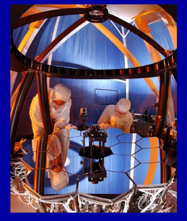
Ball 1/6-scale model: WFS produces diffraction-limited images at 2.0  $\mu$ m.
