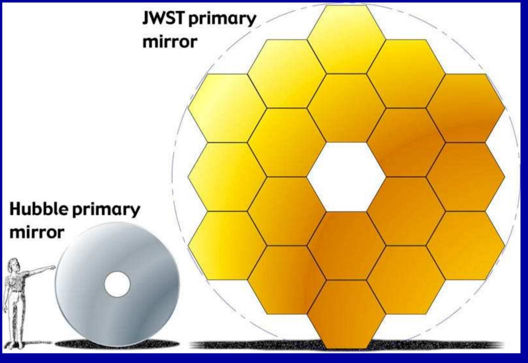
JWST  $\sim 2.5 \times$  larger than Hubble, so at  $\sim 2.5 \times$  larger wavelengths: JWST has the same resolution in the near-IR as HST in the optical.
