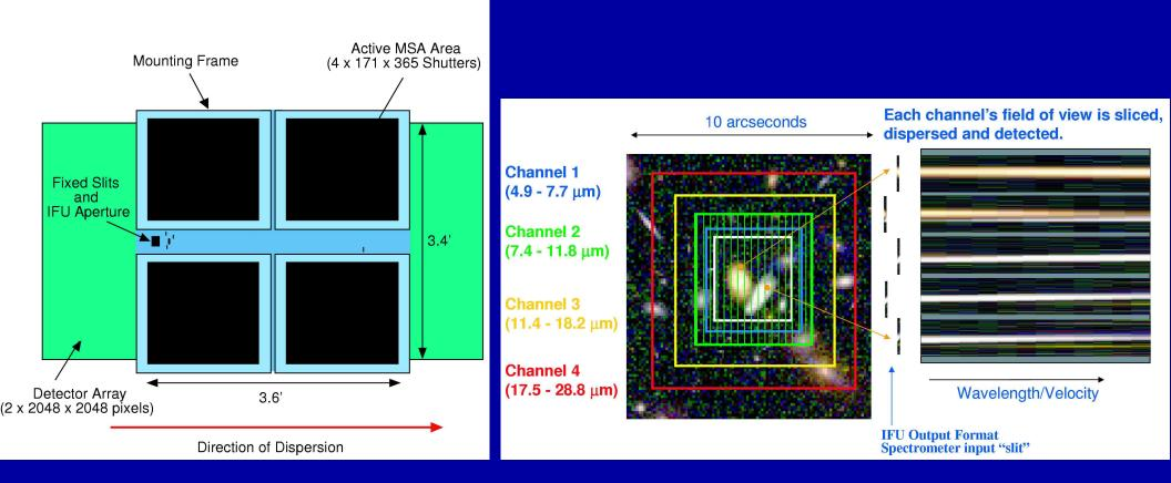
JWST offers significant multiplexing for faint object spectroscopy:
