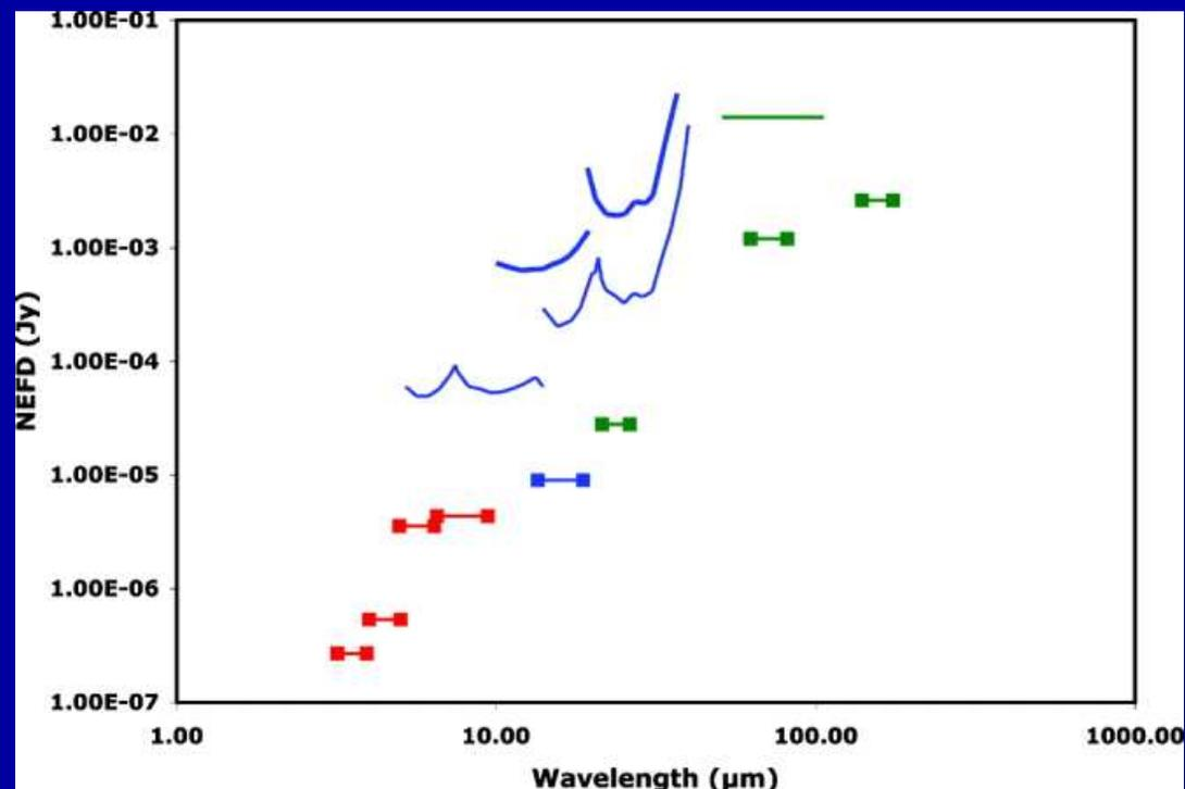
Fig. 3.— Point-source sensitivity and wavelength coverage of the *Spitzer* science instruments.
