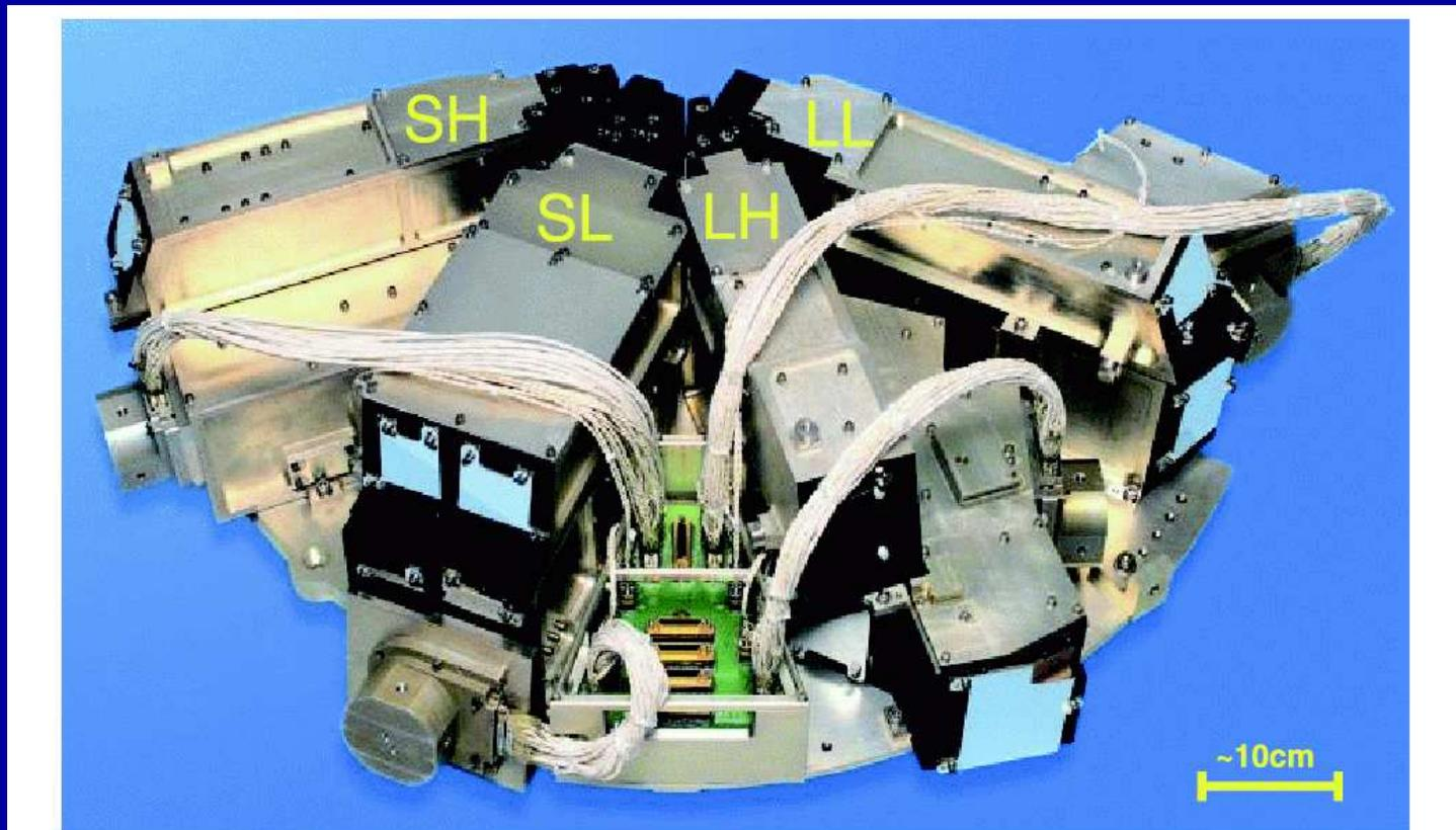
FIG. 1.—Infrared Spectrograph on *Spitzer*. The four IRS modules, SH, SL (which includes the peak-up cameras), LH, and LL are marked. A schematic of the location of the spectrograph slits on the *Spitzer* focal plane is presented in Fig. 2 of Werner et al. (2004).
