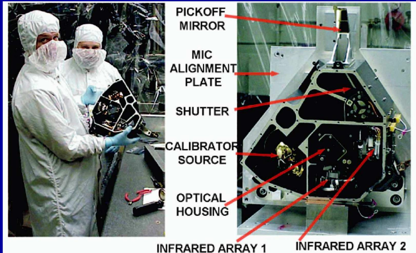
Fig. 1.— IRAC Cryogenic Assembly (CA) at NASA GSFC, with the top cover removed to show the inner components. The parts marked Infrared Array 1 and 2 are the IRAC channel 4 and 2 focal plane assemblies, respectively.
