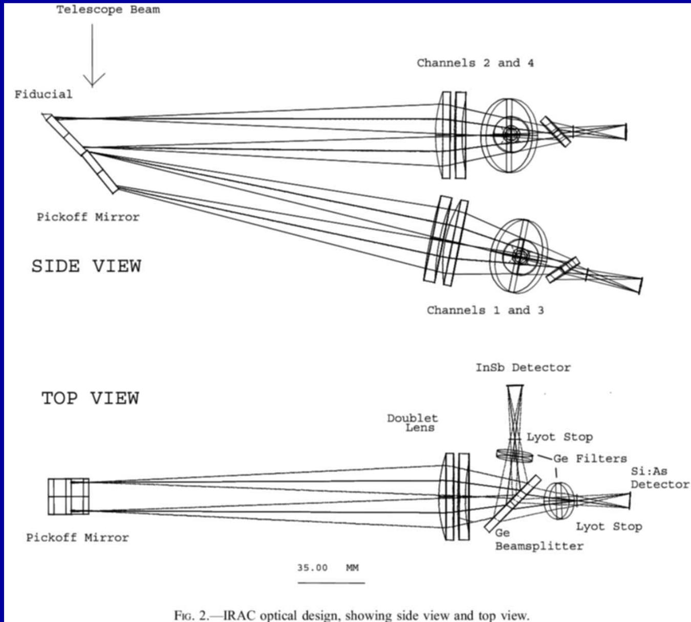
FIG. 2.—IRAC optical design, showing side view and top view.
