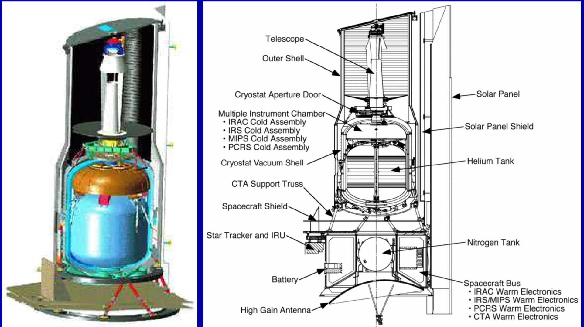
Fig. 1. — Cutaway view of the *Spitzer* flight hardware. The observatory is approximately 4.5 m high and 2.1 m in diameter. The dust cover is shown prior to its ejection approximately 5 days after launch.
